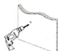
Step 2: Punch holes at the marked positions with an electric drill, the depth of which is the length of the expanded rubber cap.
