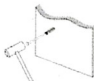
Step 4: Nail the screw into the expanded rubber cap with the nail head reserved for 5mm and hang the product back hook on the screw to finish.
